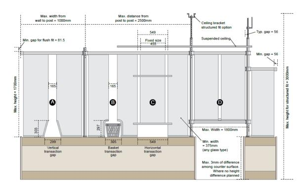
Sample elevation to illustrate available transaction gap types, upper fixing styles and system limitations.
